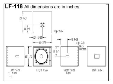
hardware recessed to be flush with the exterior of the enclosure. A 16gauge carbon steel epoxy coated grill shall be utilized for transducer protection. An integral steel socket shall be included to facilitate and the mounting of satellite speaker systems via an optional 1.5" diameter pole. The input panel shall be removable via a field connector system to facilitate servicing and exchange of input panels. The loudspeaker system shall be the OAP Audio product model LF-118.
