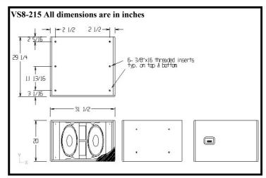
Six flying points shall be incorporated on each side of the cabinet. The loudspeaker shall be the OAP Audio model VS8-215.
