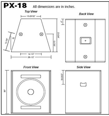
The usable frequency response of the system shall be from 45 Hz to 200 Hz. Axial sensitivity of the loudspeaker shall be 96.75 dB, 1 watt at 1 meter. The loudspeaker shall be the OAP Audio PX-18. NOTE: As a research and development corporation, OAP Audio reserves the right to change specifications to improve performance.
