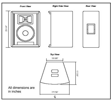
a 1" compression driver mounted on a defined coverage horn. The system shall have a frequency range of 65 Hz to 16,000 Hz, a pressure sensitivity of 104 dB at 1 watt power capacity giving a maximum output capability of 123 dB measured at 1 meter and averaged between 125 Hz and 8,000 Hz. The cabinet shall be constructed of void-free 3/4" birch plywood and stiffened internally. All exposed corners shall be rounded for damage resistance. The system shall be the OAP MT-122.
